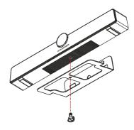
5. Slide the fixed device bracket onto the wall bracket.
